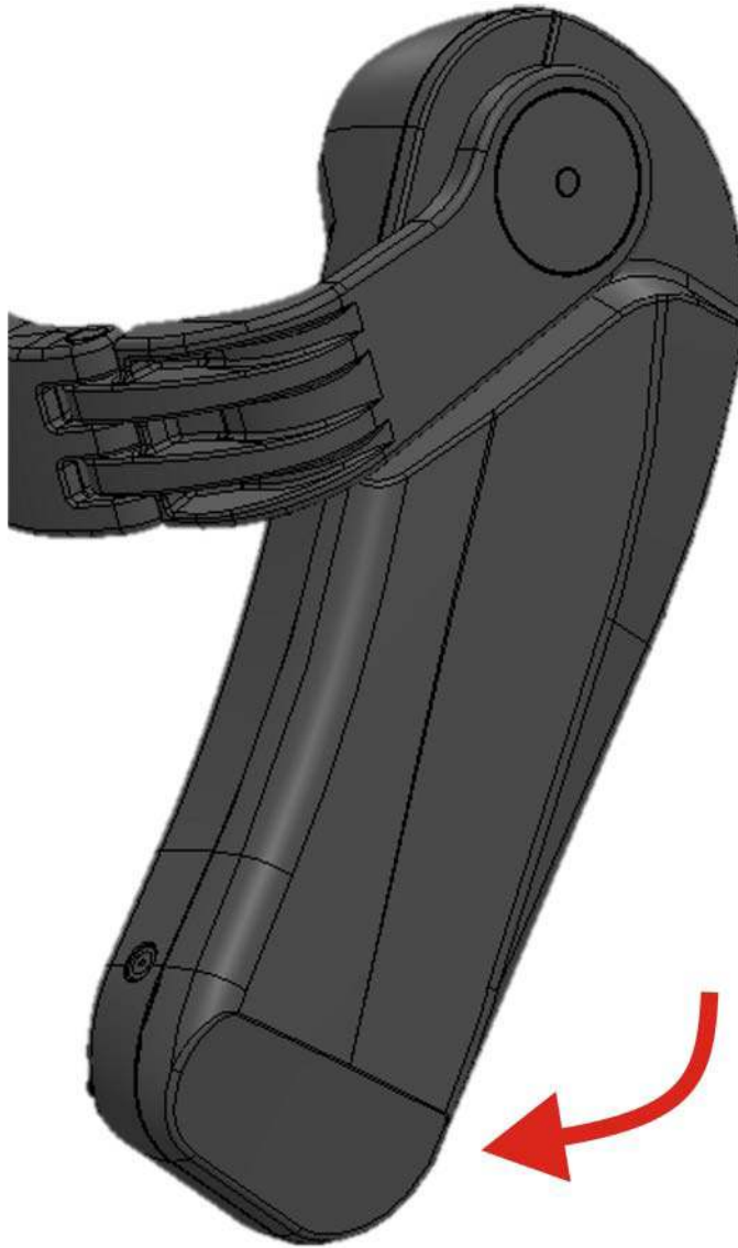
Fig. 2.6 - Torque Generator Box in rear rest position. This is the only position where the locking mechanism can be activated or deactivated
