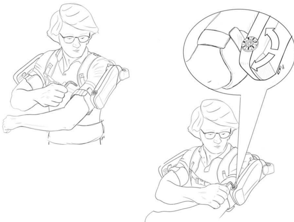
Fig. 3.7 - Assistance level operating principle
