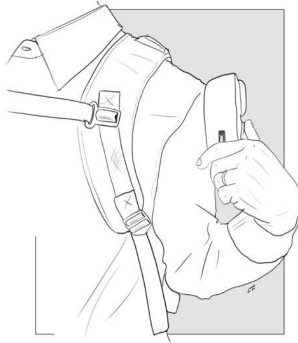
Fig. 3.13 - Unlocking the locking mechanism of the Torque Generator Box.
