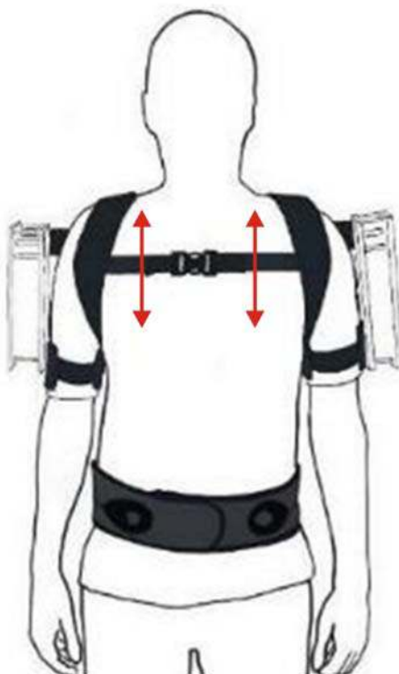
Fig. 3.5 - Operating principle of the front buckle adjustment
